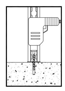
2) DRILL A 1/2" DIAMETER HOLE THROUGH FOOTPLATE AND INTO CONCRETE. THE HOLE SHOULD BE 1/2" DEEPER THAN THE LENGTH OF THE FLOOR ANCHOR.
