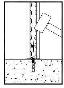
3) USING A HAMMER TAP THE PREASSEMBLED ANCHOR THROUGH THE FOOTPLATE AND INTO THE HOLE. NOTE: PREASSEMBLE ANCHOR SO THE NUT IS SLIGHTLY ABOVE THREADS. THIS PREVENTS DAMAGE TO THREADS WHILE HAMMERING THE FLOOR ANCHOR INTO THE HOLE. THE ANCHOR SHOULD BE SEATED FIRMLY AGAINST THE FOOTPLATE.
